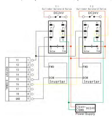
**2. Count 3, multi-speed:** One spindle with one inverter, spindle 3,4 same as 1,2.
