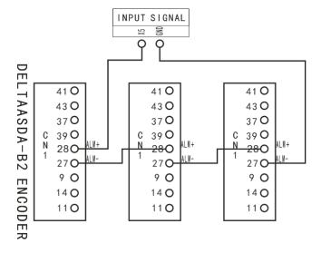
Alarm signal normal open, wiring in parallel
