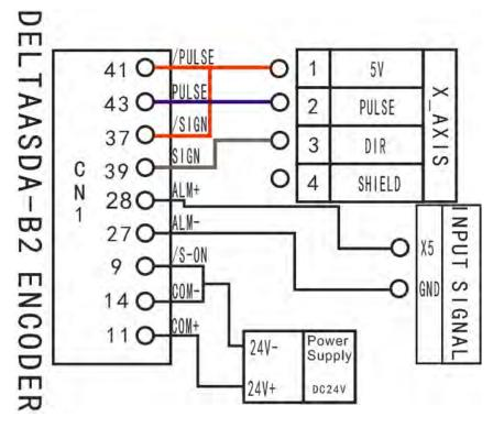
A2 Series PULSE,/PULSE,SIGN,/SIGN correspond pin-43,41,36,37, COM- corresponds pin-45/47/49
