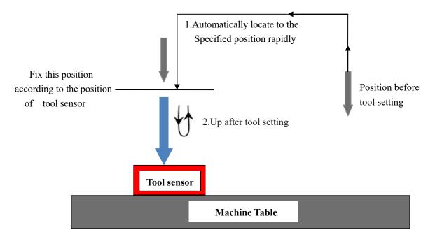
Fixed calibration refers to measurement operation at a certain fixed position on the machine.
