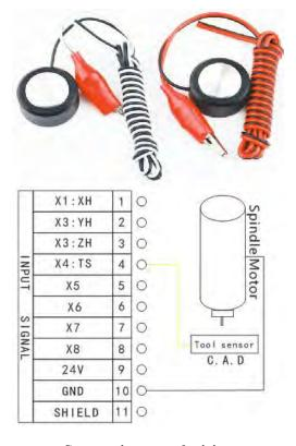
Sensor picture and wiring
