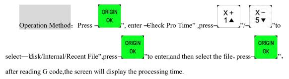
CAUTION: Plesae pull out the U disk correctly after copying files from computer, if not, the controller may not recognize the U disk.
