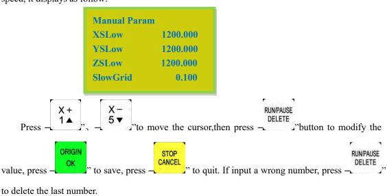
In order to ensure the accuracy of processing and debugging, the system introduces the concept of grid which also called minimum feed. It range is 0.05mm-1.0mm. When user change mode to —tep", machine will move by grid distance.
